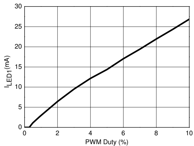
LED Current (AL1782) vs. PWM Duty (f=500Hz, 0~10%)
