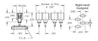
Interconnect Socket Surface Mount Socket Accepts .015"- .025" (0,38 - 0,635 mm) dia leads Single Row Surface Mount **Plating Code:** 41 Shell Plating: 200 µ" Tin (matte finish) over 100 µ" Nickel Inner Contact Plating:
