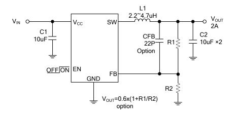
$V_{OUT}$ = $V_{FB}$  × (1+R1/R2),  $V_{FB}$ =0.6V, R2 suggest 60k $^{\sim}$ 300k $\Omega$
