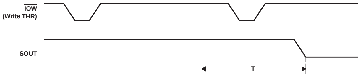
Figure 22. Error Case Timing Condition
