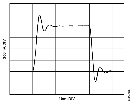
Figure 35. Small Signal Transient Response, G = 12.04 dB
