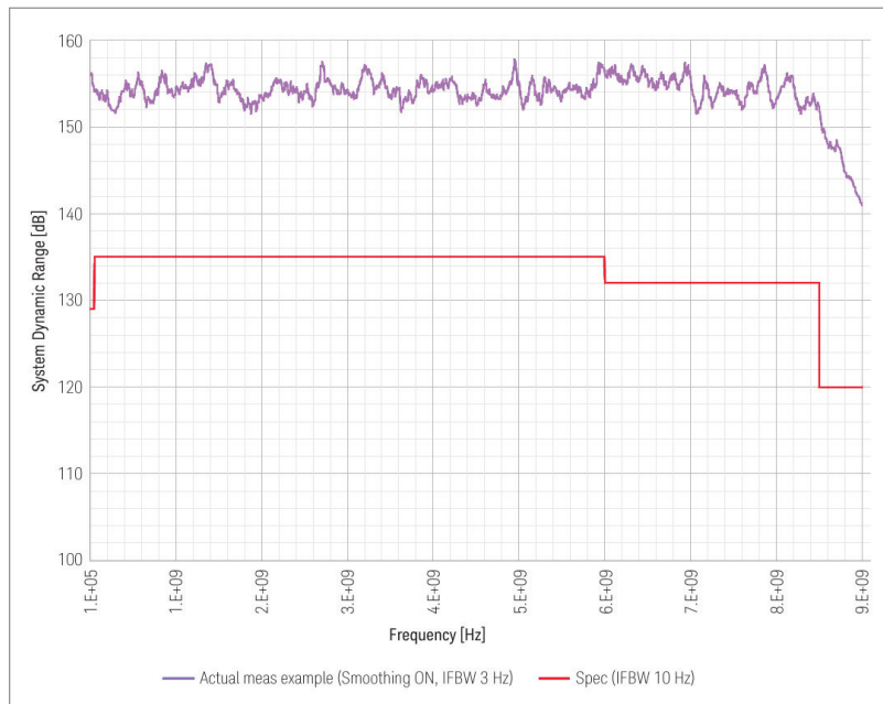
System dynamic range (specification and actual measurement data example)
