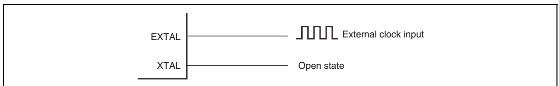
Figure 4.4 Example of External Clock Connection
