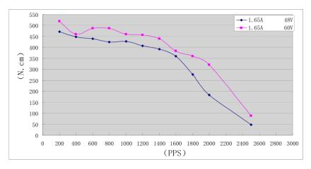
Motor model: 86BYGH450B-001 Driver model: SD-2H086MB
