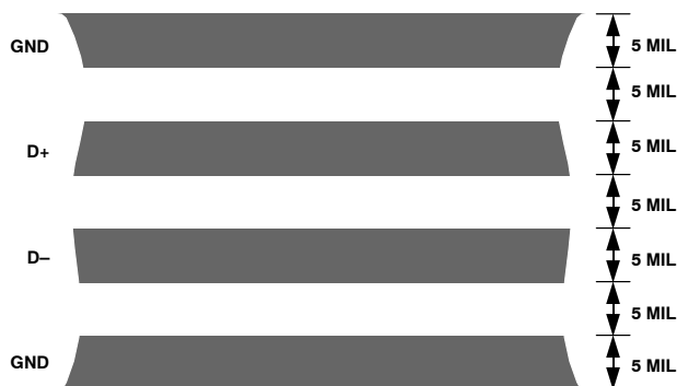
Figure 22. Typical Arrangement of Signal Tracks
