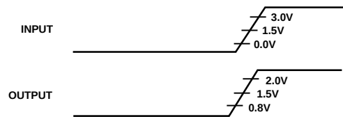
Figure 28. Voltage Reference Levels for AC Measurements (Except Output Enable/Disable)
