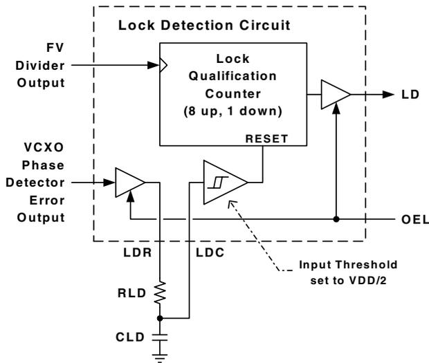
If the lock detection circuit is not used, the LDR output may remain unconnected, however the LDC input should be tied high or low. If the PCB was designed to accommodate the RLD and CLD components but the LD output will not be used, RLD can remain unstuffed and CLD can be replaced with a resistor ( $< 10 \text{ kohm}$ ).
