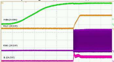
Startup through PV IN 1A Load, V IN =5.5V
