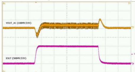
Load Transient (V IN =3.8V, PWM, I O =0A to 1A)
