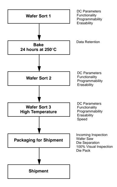
Figure 1. AMD KGD Product Test Flow
