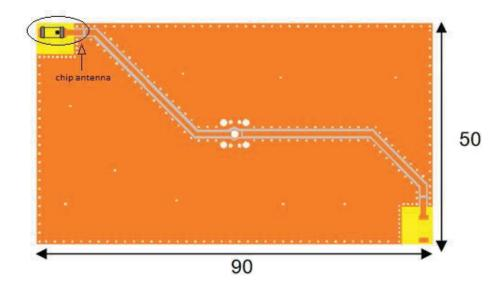
Evaluation Board dimension: 90 x 50 mm Unit: mm
