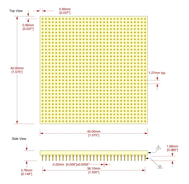
Substrate: 1.59mm ±0.18mm [0.0625" ±0.007"] FR4/G10 or equivalent high temp material.
