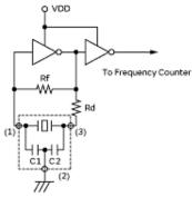
Regarding CERALOCK® with built-in capacitors, the terminal (1) and (3) are interchangeable, but if connection is interchanged, the specification of initial tolerance frequency may not be guaranteed. \*Please see dimensions about terminal numbers.
