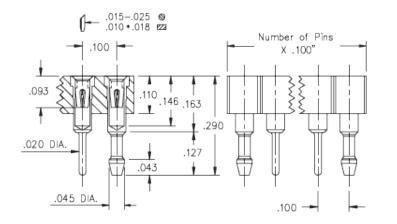
Description: Interconnect Socket Solder Tail Socket with Clinch Pin Retention Pins Accepts .015"- .025" (0,38 - 0,635 mm) dia leads Single Row Through Hole Plating Code: 43 Shell Plating: 200  $\mu$ " Tin (matte finish) over 100  $\mu$ " Nickel Inner Contact Plating: 30 µ" Gold over 50 µ" Nickel
