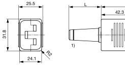
1) Cut cable guard to suit cable diameter
