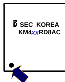
b. Top marking example of normal package
