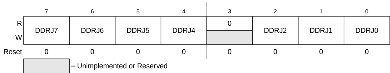
Figure 22-58. Port J Data Direction Register (DDRJ)
