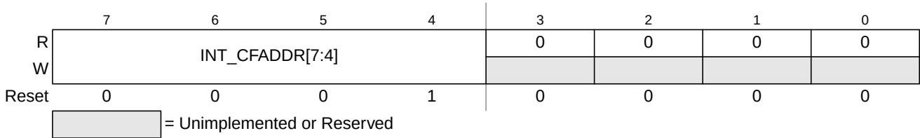
Figure 16-5. Interrupt Configuration Address Register (INT_CFADDR)
