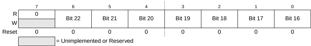
Figure 20-15. Debug Comparator Address High Register (DBGXAH)
