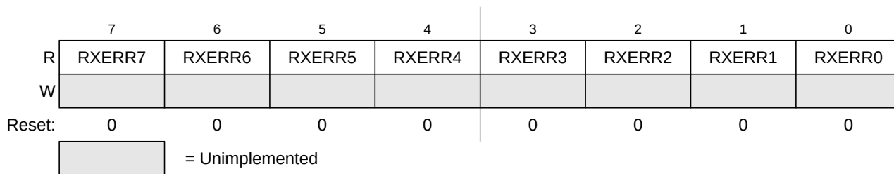
Figure 10-18. MSCAN Receive Error Counter (CANRXERR)
