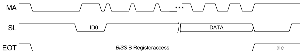
Figure 13: BiSS B register access (EN_MO = 0)
