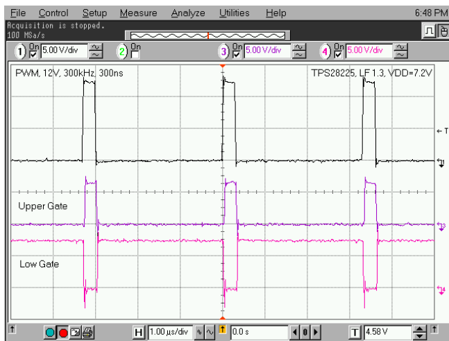
Figure 22. 12-V PWM Pulse at V_{DD} = 7.2 V
