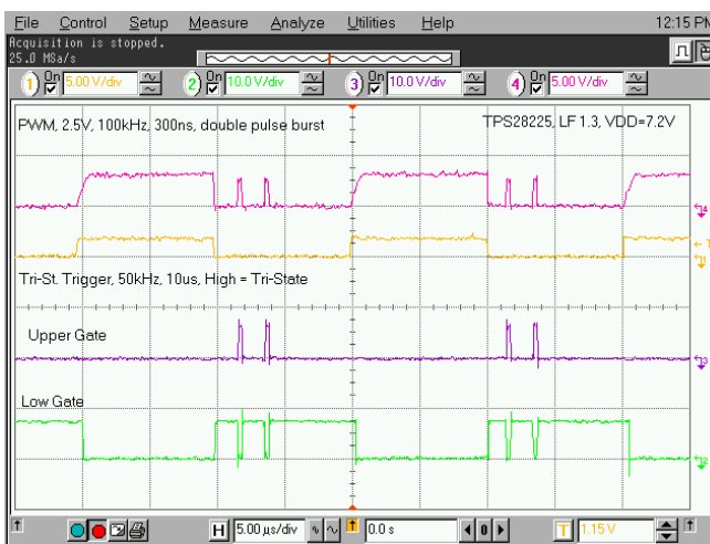
Figure 21. 2.5-V Amplitude PWM Pulse (TPS28225)
