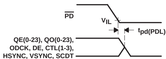
Figure 7. Delay From \overline{\text{PD}} Low to Hi-Z Outputs
