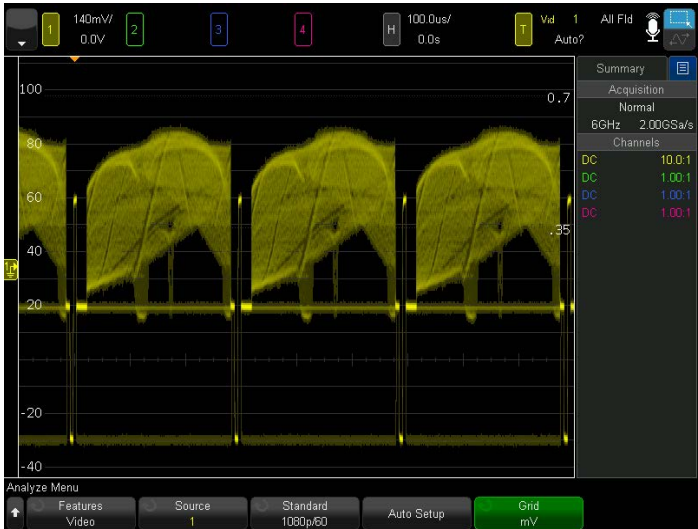
Figure 45. Triggering on a 1080p/60 signal.
