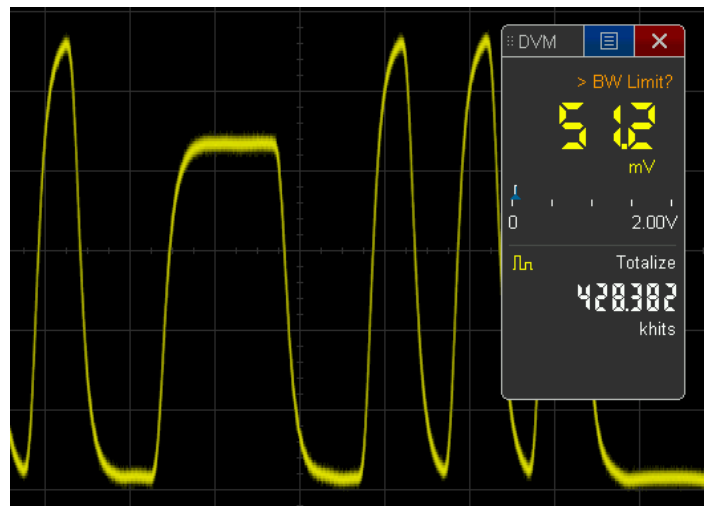
Figure 35. Totalizing the number of runt errors.
