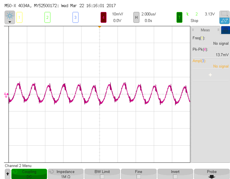
Figure 8. Measured Output Voltage Ripple at 12V Voltage Input, 3.3V/25A, f_{SW} = 600\text{kHz} , Measured Across C_{OUT2} Using 1 \times Probe
