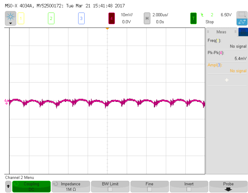
Figure 7. Measured Output Voltage Ripple at 12V Voltage Input, 1.5V/25A, f_{SW} = 600\text{kHz} , Measured Across C_{OUT6} Using 1 \times Probe
