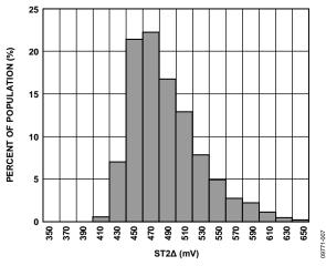
Figure 13. ST2 Output Change at 25°C ( $V_{RATIO} = 5 V$ )
