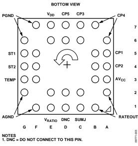
Figure 3. Pin Configuration
