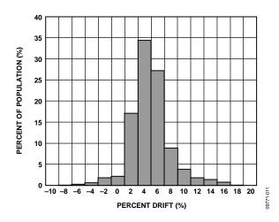
Figure 8. Sensitivity Drift over Temperature
