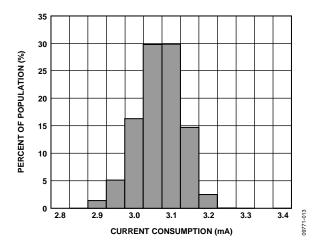
Figure 18. Current Consumption at 25°C ( $V_{RATIO} = 5 V$ )
