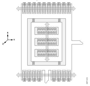
Figure 19. Simplified Gyroscope Sensing Structure—One Corner
