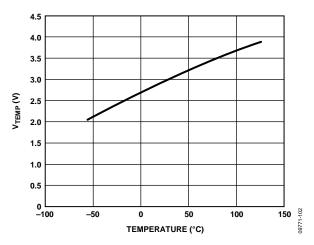
Figure 17.  $V_{TEMP}$  Output vs. Temperature
