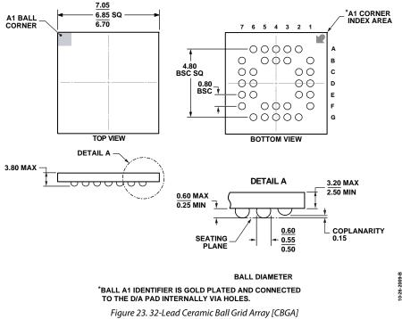
Figure 23. 32-Lead Ceramic Ball Grid Array [CBGA] (BG-32-3) Dimensions shown in millimeters
