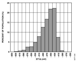
Figure 10. ST1 Output Change at  $25^{\circ}$ C ( $V_{RATIO} = 5 V$ )
