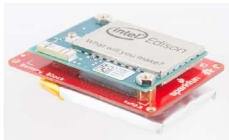
Battery Block Installed
