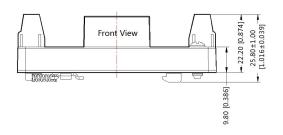
Note: Unit: mm[inch] Mounting rail: TS35 Wire range: 24-12 AWG
