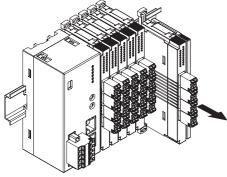
• Removing an intermediate module
