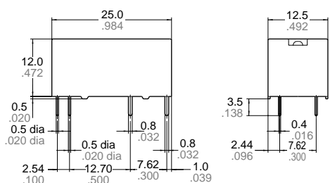
2 coil latching type
