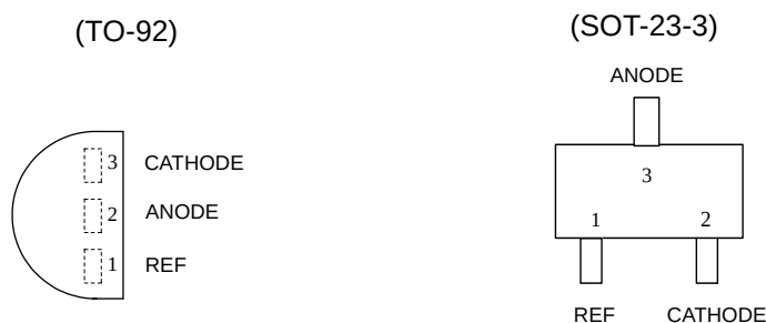
Figure 2. Pin Configuration of BM431 (Top View)
