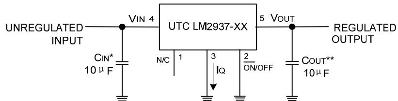
\* Required if the regulator is located more than 3 inches from the power supply filter capacitors.
