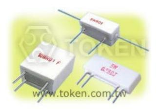
The four terminal resistors are a new version of Token's (LSQ) Current Sense Family Series which was specially designed for use in a Kelvin configuration where a current is applied through two opposing leads and sensing voltage is measured across the other two leads. Token LSQ series is specifically designed for low resistance applications requiring the highest accuracy and temperature stability.
