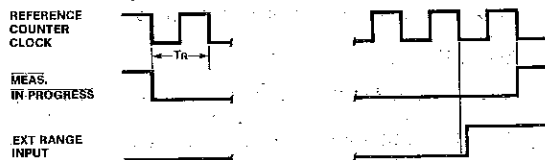
Figure 4: External Range Input to End of Measurement in Progress.
