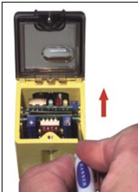
Figure 6. Using the small screwdriver in the module slot if necessary to nudge the module loose, lift the module up and out.
