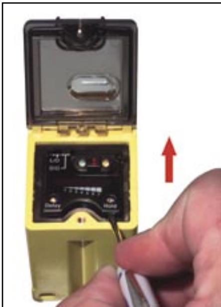
Figure 5. Insert a small screwdriver into the slot and lift the black cover to remove.
