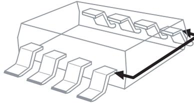
**Clearance:** The shortest distance between two conductive input to output leads measured through air (line of sight).
