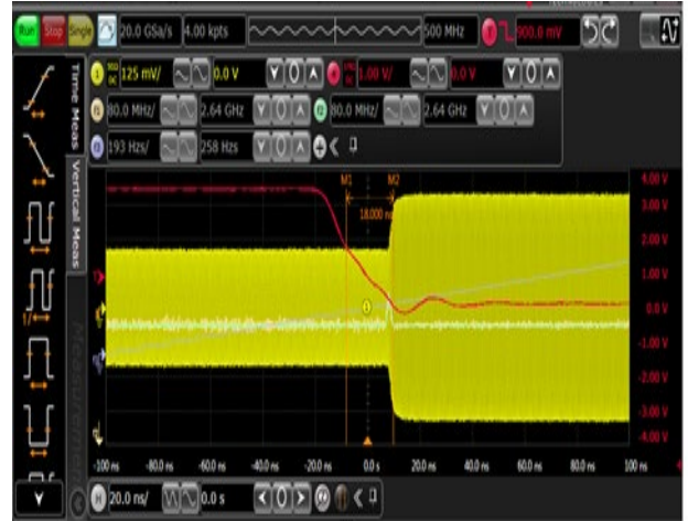
Figure 22. Power ON Switching Time
