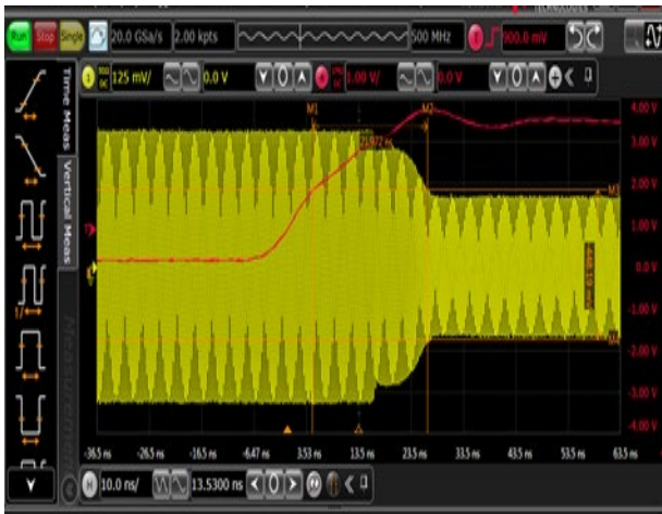
Figure 21. Power OFF Switching Time
