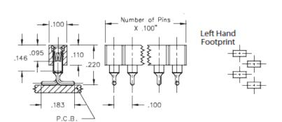
**Description:** Interconnect Socket Surface Mount Socket Accepts .015" - .025" (0,38 - 0,635 mm) dia leads Single Row Surface Mount **Plating Code:** Shell Plating: 200 μ" Tin/Lead(93/7) over 100 μ"
