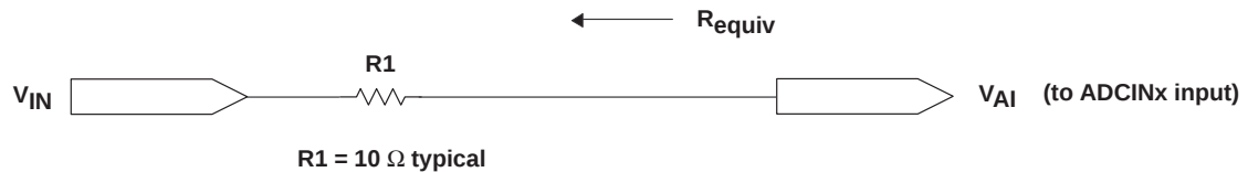
Figure 42. Typical ADC Input Pin Circuit
