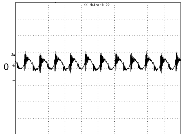
Figure 11: Input Terminal Ripple Current, i_c , at full rated output current and nominal input voltage with 12\mu H source impedance and 33\mu F electrolytic capacitor (200 mA/div, 2us/div).
