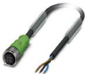
Sensor/actuator cable, 3-position, PUR halogen-free, black-gray RAL 7021, free cable end, on Socket straight M12, coding: A, PIN 2+4 bridged, cable length: 5 m
