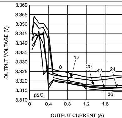
Figure 24. Line and Load Regulation,  $T_A = 85^\circ\text{C}$
