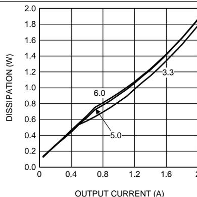
Figure 20. Dissipation 36-V Input,  $T_A = 85^\circ\text{C}$
