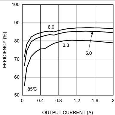
Figure 19. Efficiency 36-V Input,  $T_A = 85^\circ\text{C}$
