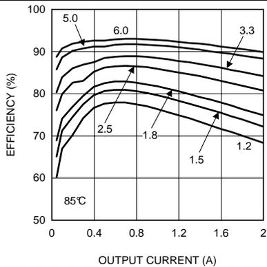
Figure 15. Efficiency 12-V Input,  $T_A = 85^\circ\text{C}$
