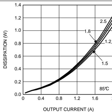
Figure 12. Dissipation 6-V Input,  $T_A = 85^\circ\text{C}$
