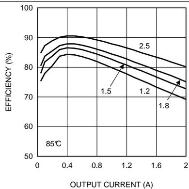
Figure 11. Efficiency 6-V Input,  $T_A = 85^\circ\text{C}$
