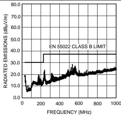
**Figure 37. Radiated Emissions (EN 55022 Class B)
