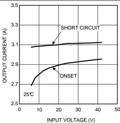
**Figure 29. Current Limit,  $V_{OUT} = 3.3\text{ V}$ ,**
