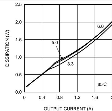
Figure 22. Dissipation 42-V Input,  $T_A = 85^\circ\text{C}$
