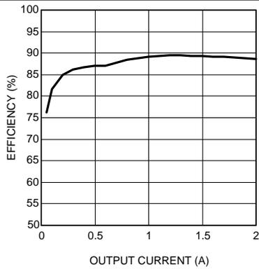
**Figure 35. Efficiency  $V_{IN} = 24\text{ V}$   $V_{OUT} = 5\text{ V}$**
