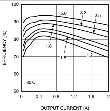
Figure 13. Efficiency 8 V Input,  $T_A = 85^\circ\text{C}$
