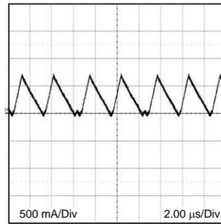
**Figure 34. Transition Mode Operation**
