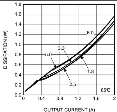
Figure 18. Dissipation 24-V Input,  $T_A = 85^\circ\text{C}$
