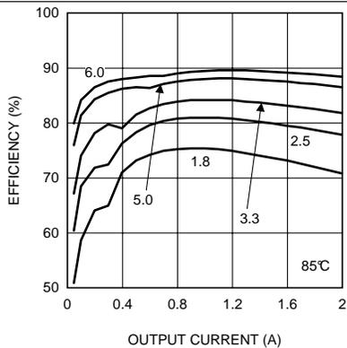
Figure 17. Efficiency 24-V Input,  $T_A = 85^\circ\text{C}$
