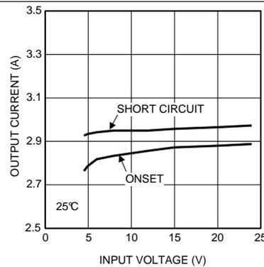
**Figure 28. Current Limit,  $V_{OUT} = 3.3\text{ V}$**
