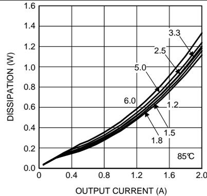
Figure 16. Dissipation 12-V Input,  $T_A = 85^\circ\text{C}$
