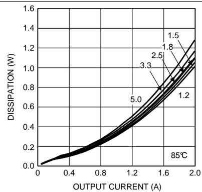
Figure 14. Dissipation 8-V Input,  $T_A = 85^\circ\text{C}$
