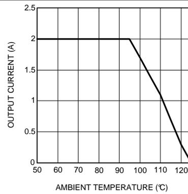
**Figure 36. Thermal Derating Curve
