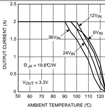
**Figure 27. Thermal Derating,  $V_{OUT} = 3.3\text{ V}$**
