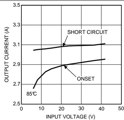
**Figure 30. Current Limit,  $V_{OUT} = 3.3\text{ V}$ ,  $T_A = 85^\circ\text{C}$**
