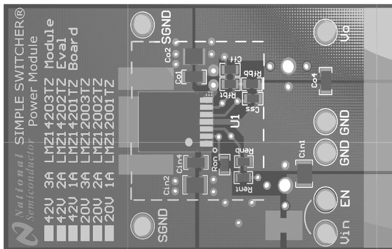
Figure 40. EVM Board Layout - Top View
