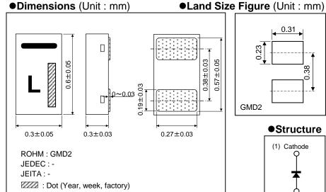
Structure (1) Cathode (2) Anode
