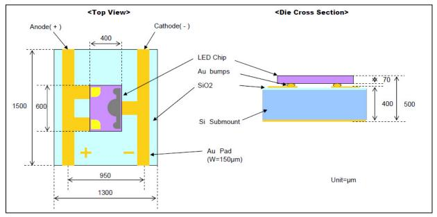
Solder (Au-Sn) or Resin (Ag) is recommended for bonding of the submount
