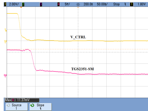
Switching Speed - Off 50 ns V_c = 0/-40\text{ V} , Freq = 3 GHz, Pin = 30 dBm, +25 °C
