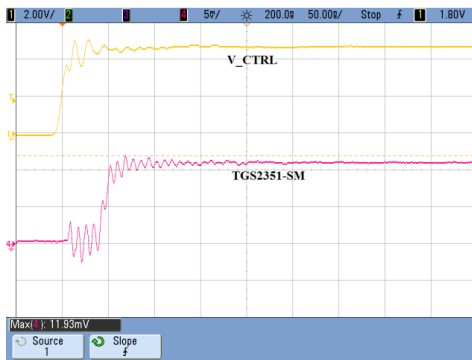
Switching Speed – On 50 ns V_c = 0/-40\text{ V} , Freq = 3 GHz, Pin = 30 dBm, +25 °C
