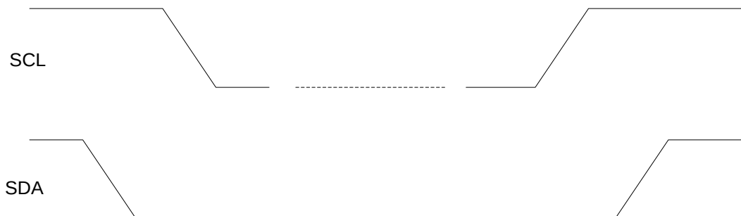
Figure 6: I 2 C START and STOP Condition Timing
