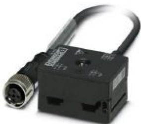
AS-Interface distributor with a high degree of protection, for a branch from two flat-ribbon conductors to a 1.0 m PUR round cable with straight M12-SPEEDCON socket
