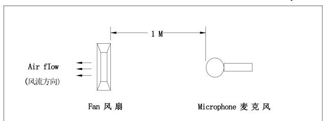
(在背景噪音不超过 18dB ( A ) 的无响室内,将待测风扇通入额定的工作电压,悬掉入空中,将麦克风放于风扇同一平面且离待测风扇进风口一米处进行测试其 B&K 值 ) Noise is measured rated voItage in free air in anechoic chamber with B&K sound IeveI meter with microphone at a distance of one meter from the fan intake.The background noise is 18Db(A) max。
