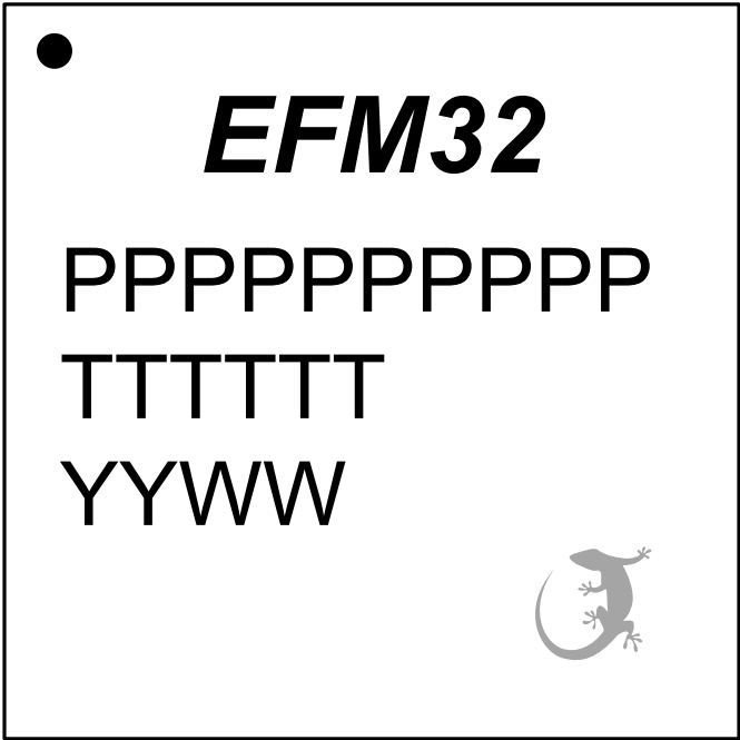
Figure 11.3. TQFP64 Package Marking
