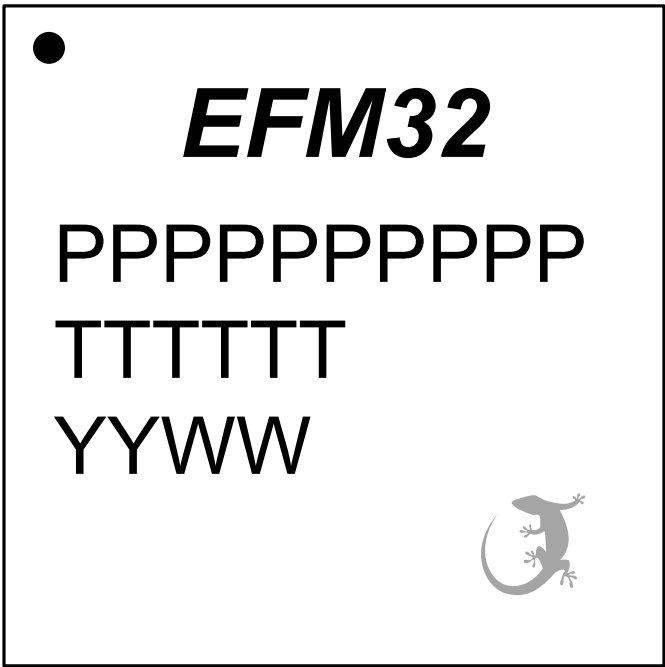
Figure 10.3. TQFP100 Package Marking
