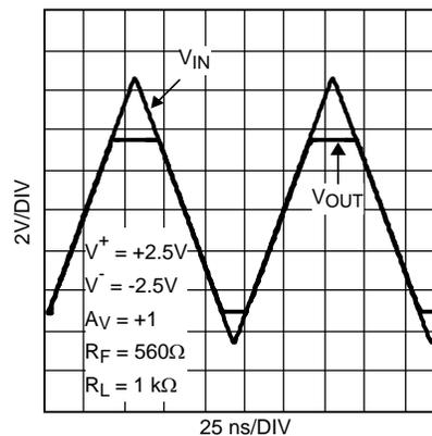
**Figure 66. Input and Output Shown with CMVR Exceeded**
