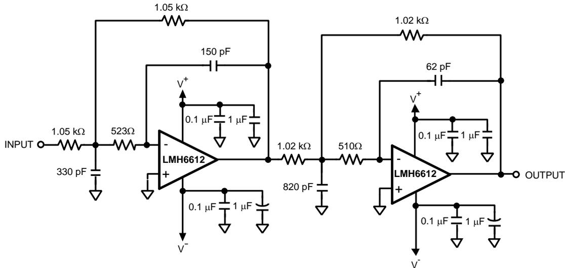
Figure 75. 4<sup>th</sup> Order Multiple Feedback Low-Pass Filter
